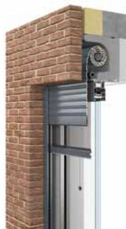
Above all, the system ensures free air circulation. The shutter box has a smaller size than the basic variant, which gives more possibilities for the external façade layer to be finished maintaining the same winding. Two revision options are available: from the inside or outside of the room, and the system can be fitted with an insect screen for extra protection against insects.
