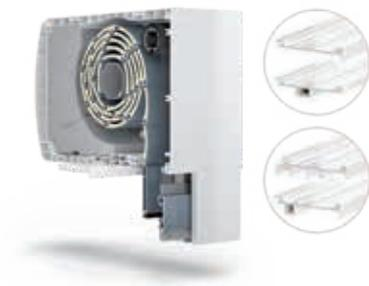
There are 7 sizes of adaptive profiles available in the offer, which enable the roller shutter box to be mounted on the window frame by clicking or sliding it from the side. These adapters work with most PVC window systems available on the market. In the case of aluminium joinery, a special distance profile with a polyamide insert can be used to install the roller shutter box. In order to minimize the occurrence of thermal bridges, it is recommended to use an expansion tape to seal the surface.
