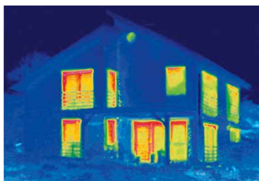
Infra-red photos – thermal imaging – clearly show where energy is lost from a house. Red indicates heat and hence high energy loss.
