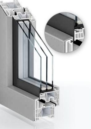
AluClip Zero – the design variant for the KÖMMERLING 76 system is available in three versions. Unique on the market, with flushmounted look and virtually flush-mounted glass pane, an all-glass look, and a classical wood and aluminium look. On this version, the glass pane in the sash lies on the same level as fixed glazing.
